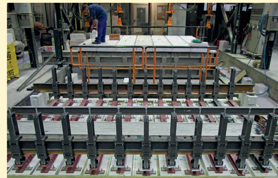
View of the testing facility before a fire test with variable joint widths
