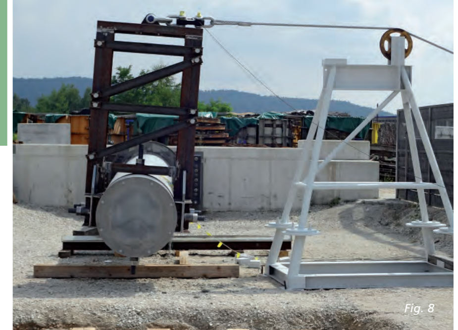
Fig. 8: Large-scale test on a spun concrete component
