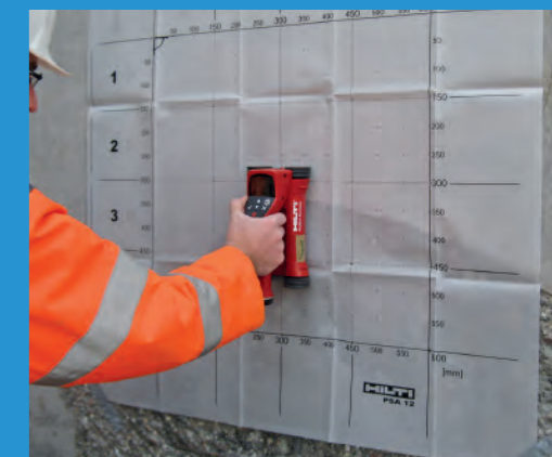
Non-destructive localisation of reinforcement
