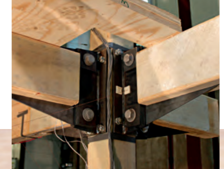
Fig. 4 (b): 3-dimensional moment connector from a previous research project (model of the 3-D frame on the earthquake table)
