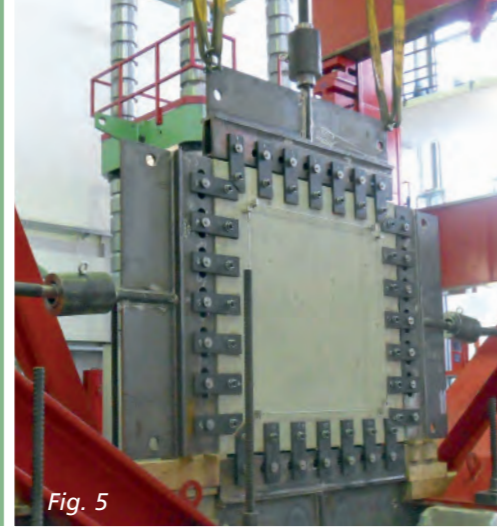
Fig. 5: Investigations on the cracking behaviour of skew reinforced concrete members
