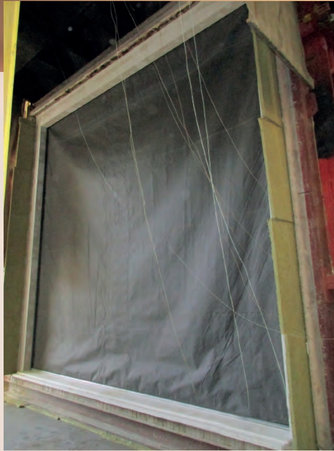
Test on an 'E90' curtain measuring (w x h) = 5000 mm x 4930 mm
