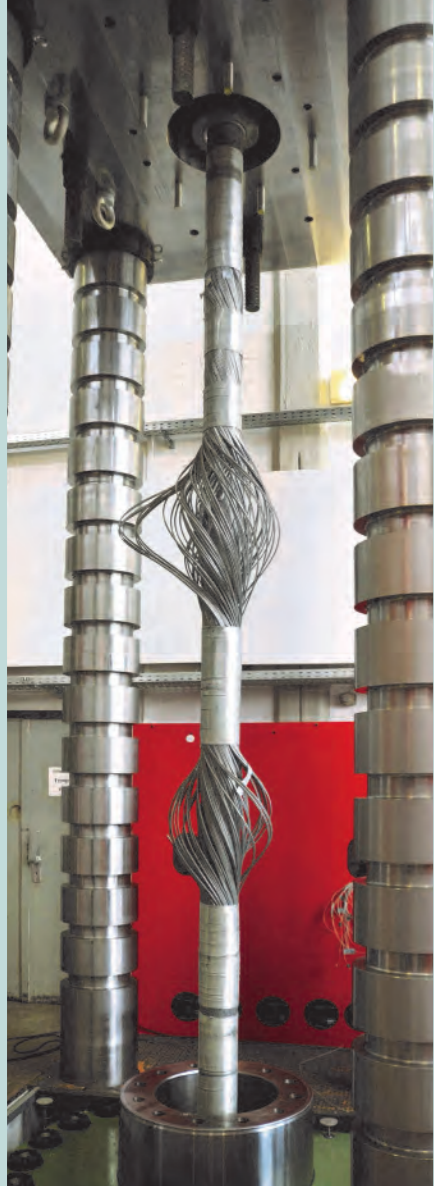
Ultimate load test on full locked cable
