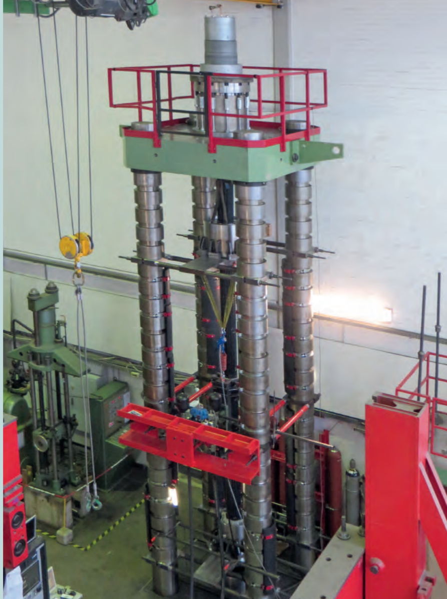
30 MN machine, axial and lateral fatigue test on stay cable system
