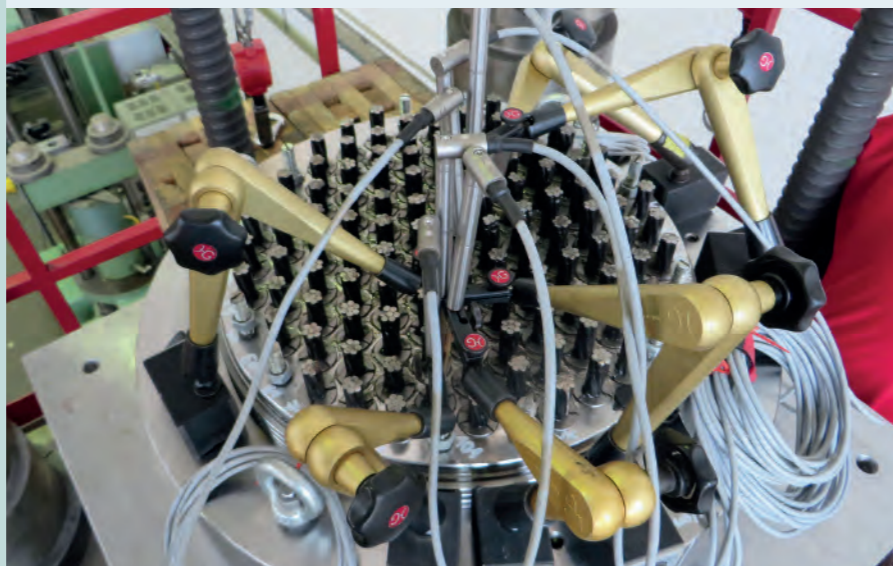
Anchorage of stay cable system with LVDT measurement
