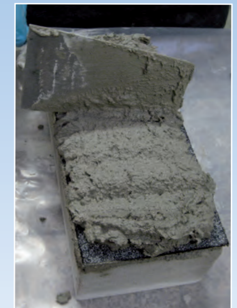
Fig. 3: Mortar bed with inserted damp-proof course
