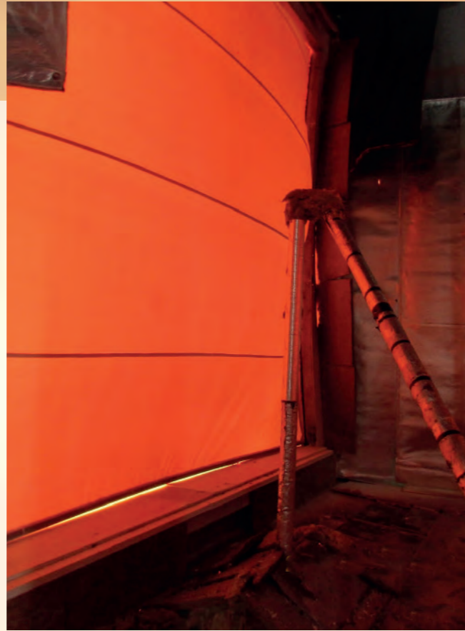
Test specimen measuring (w x h) = 5000 mm x 4930 mm in test minute 100
